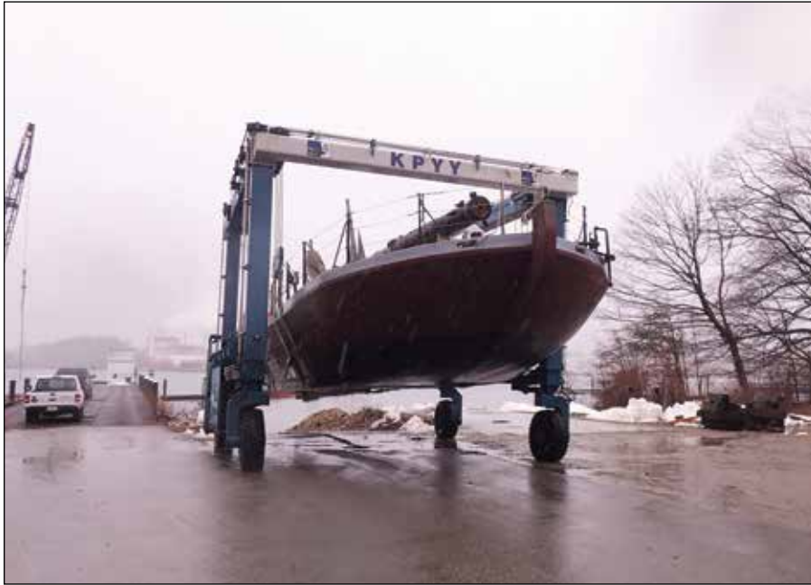
The boatyard removed its marine railway and rebuilt a deeper ramp, increasing the hauling efficiency.
